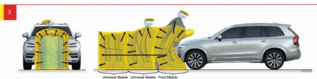
If the pressure exerted during the impact or collision is too high, the relief pressure valve is opened and allows the water to come out in a controlled manner, so part of the pressure exerted on the water is released and the contact time between the vehicle and the triple container system is longer.
