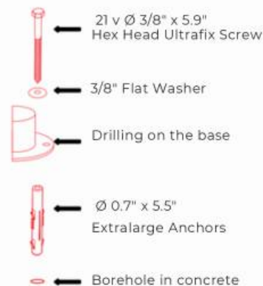
Anchoring Ø 3/8" x 5.9" Hex Head Ultrafix Screw Ø 0.7" x 5.5" Extralarge Anchor
